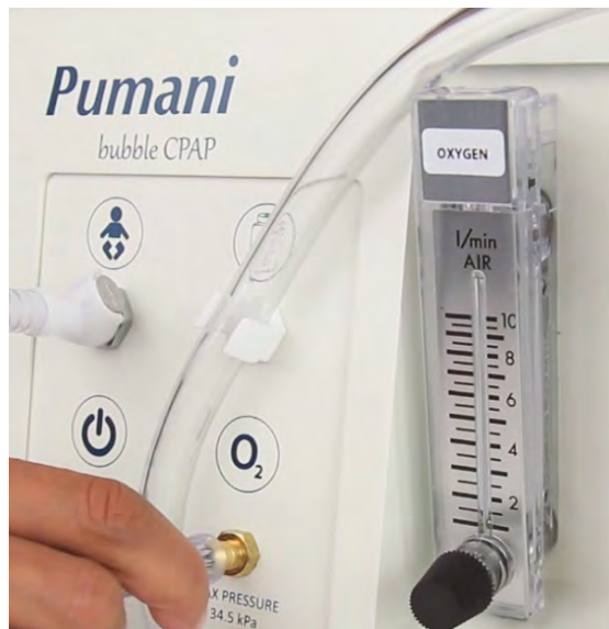
3.9 Connect Tubing to the oxygen port
