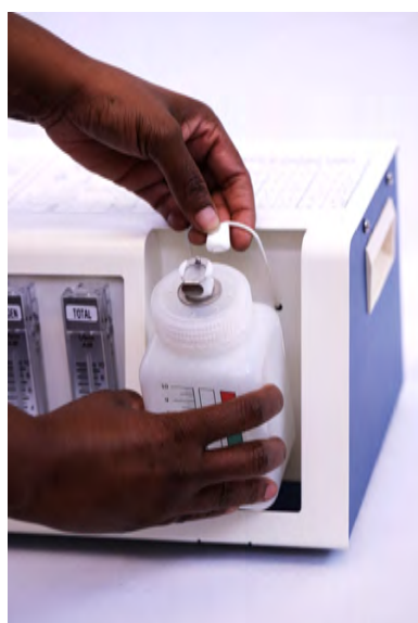
3.3 Pull bottle strap out and begin to remove bottle.
