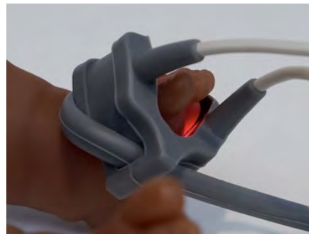
2.2 Light of pulse oximeter perfusing through skin.
