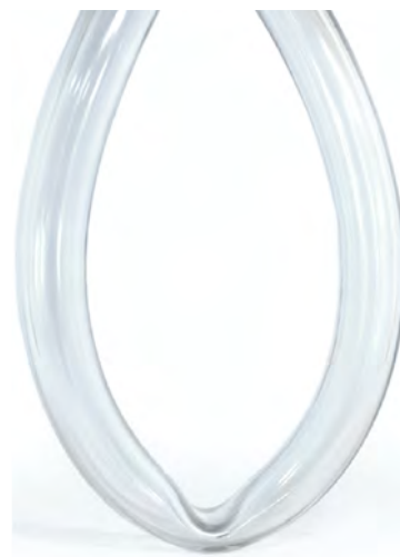
7.2 Kinks in the tubing prevent flow.
