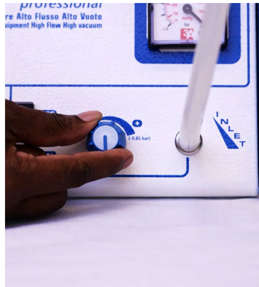
3.7 Adjust suction vacuum to desired safe level and test by suctioning water from container.
