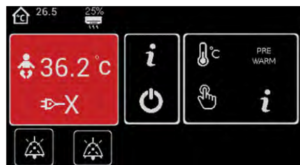
3.13 Power Failure alarm.
