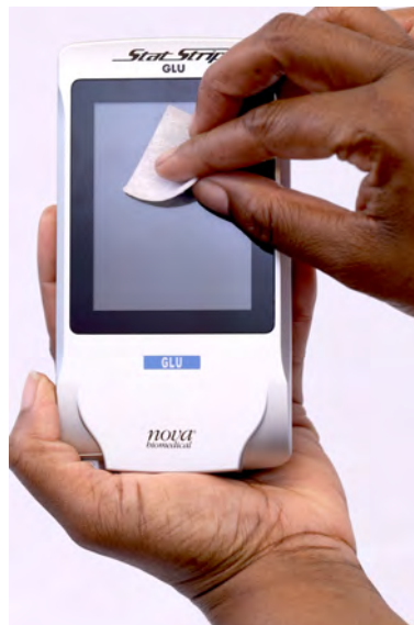
4.1 Wipe down the glucometer with 70% alcohol.
