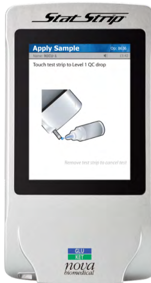
6.4 Allow the strip to absorb a drop of the control solution.
