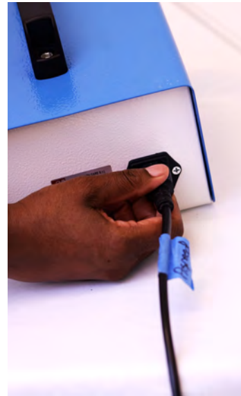
3.5 Connect power cable to device.
