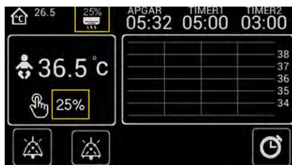
7.1b Manual settings set to 25% heat output.
