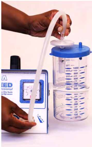
3.3 Connect short tubing to filter & inlet port.
