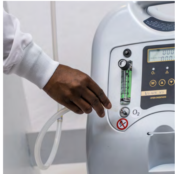
3.3 Connect correctly sized nasal prongs to oxygen port.
