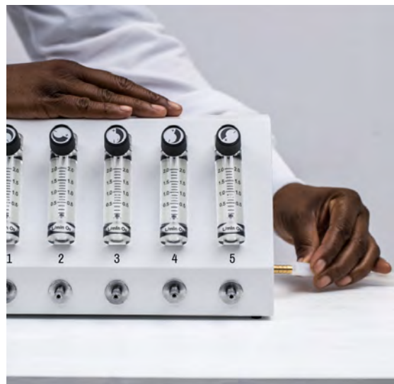
3.2 Connect flow splitter tubing from oxygen outlet to flow splitter inlet port.
