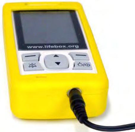
6.1 Rechargeable pulse oximeter with power port and charging cable.
